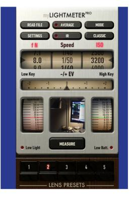
This is an accurate light meter for the occasion when you need an off-camera light meter. One situation where it might be useful is when you have a strong ND filter on and the camera meter doesn't get a reading.
